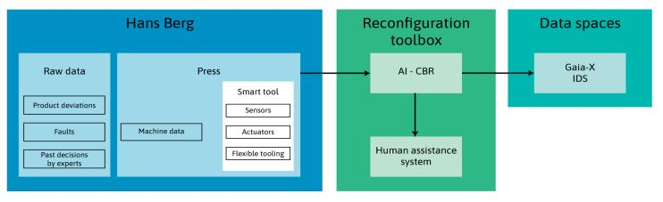
A smart tool with sensors and the recording of manual tool adjustments using human motion capture will support the adjustment measures and reconfiguration needs. Artificial intelligence (AI) will compare the information with a knowledge base that links faults to successful coordination measures.
